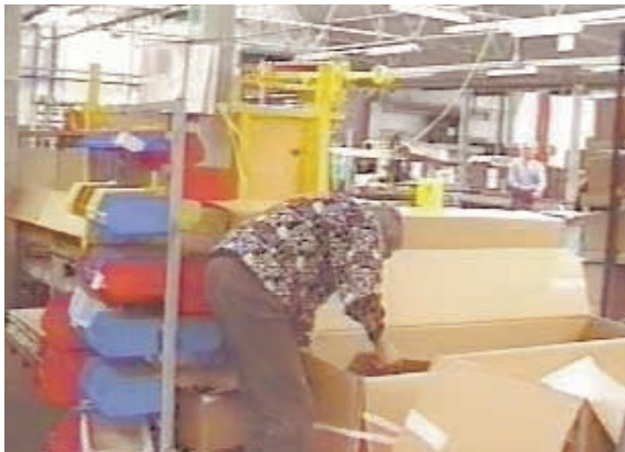
Frequent bending when picking up both heavy and light parts increases the load on the back. Picture taken from a video recording.
