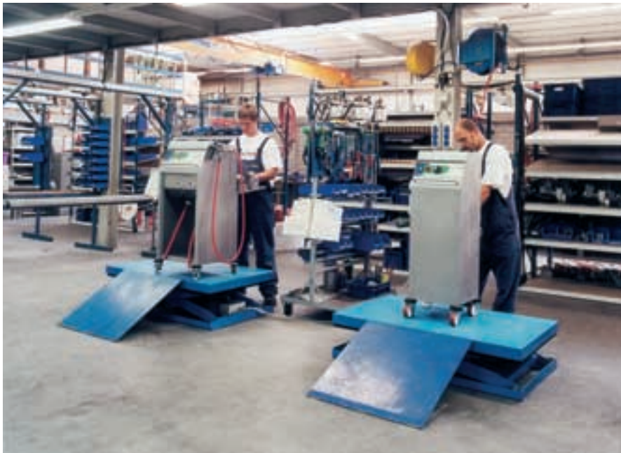
In the new situation lifting tables ensure that work can always be carried out at the correct height.
